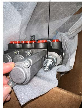
PRESSURE RELIEF VALVE WITH CAP REMOVED
